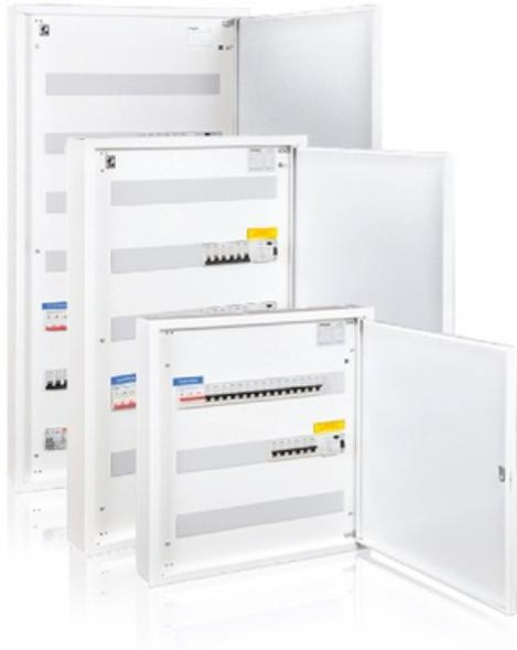
Group electric centres are suitable for use from the smallest apartments to large detached houses. The RKM and RKS electric centres are made from hot galvanised steel plate that has been painted white. The RKP electric centres are made of white plastic. The RKV group electric centres are appropriate for use as a lighting, heating or group electric centre in wet spaces. Browse our extensive and diverse selection!
